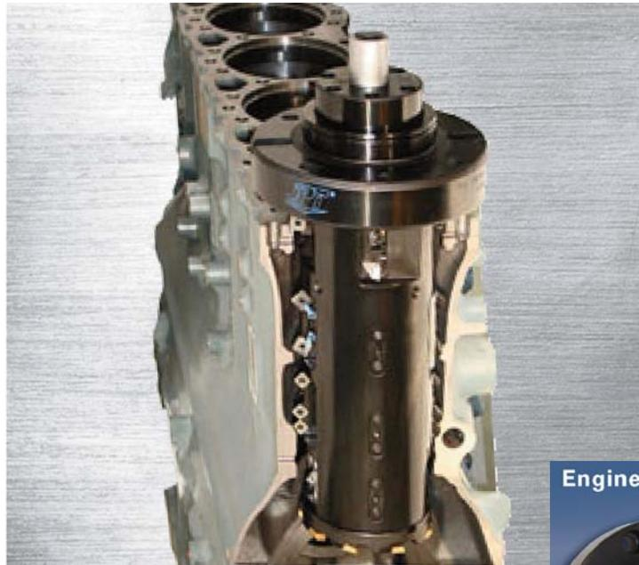
*Above: Diesel Engine Cylinder Boring with six (6) actuating slides*
